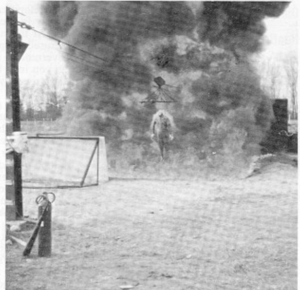
Fig. 6—Clothed mannequin being tested at Natick fire pit.
