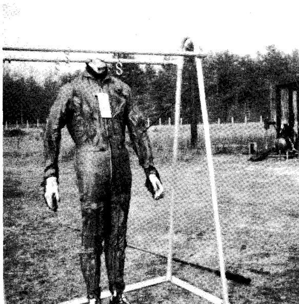
Fig. 2—PBI suit exposed to fire test.
