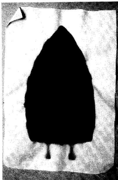
Fig. 1. Original demonstration of Thermosol dyeing process heat treatment of padded polyester fabric between two flat irons.
