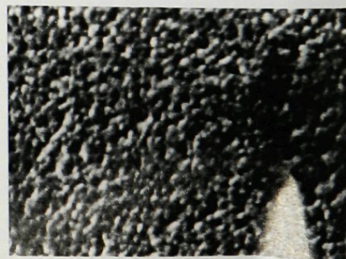
Fig. 5. Polypyrrole on glass fiber. Magnification 100,000X.
