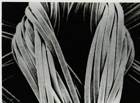
Fig. 2. Polypyrrole on knitted nylon fabric. Magnification 200X.
