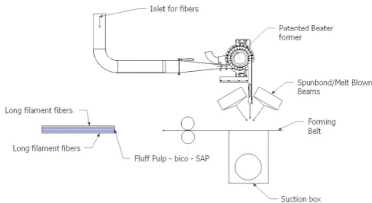
**Fig. 2.** Airlaid Campen Machinery with patent technology to create nonwoven materials.
