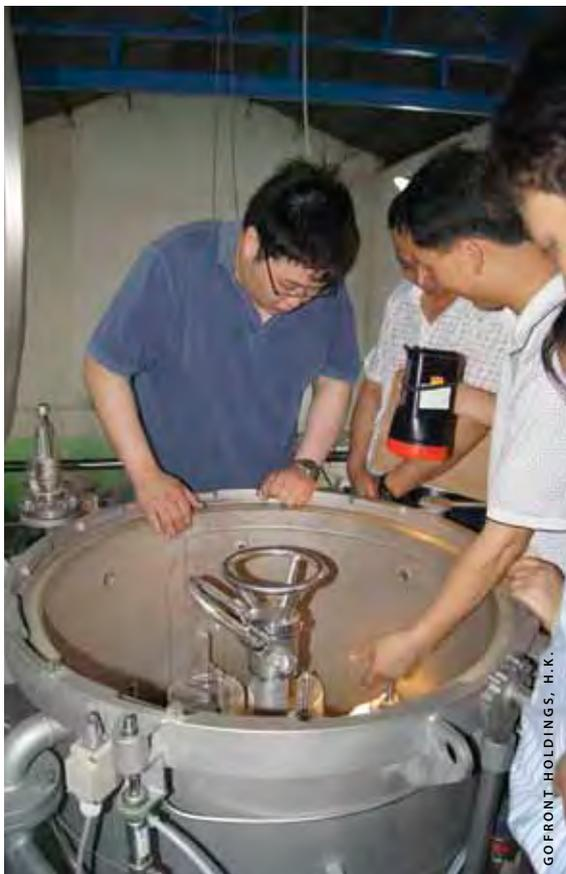
The Excel yarn dyeing machine is designed to dye with less water, a 1:2 liquor ratio.
