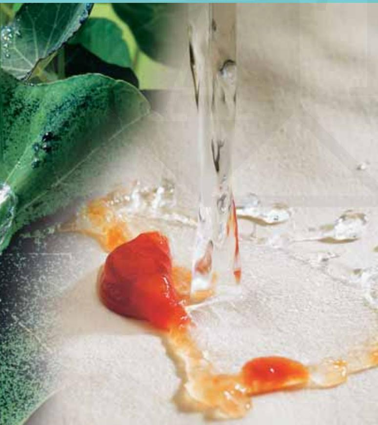
Ketchup cleans quickly on fabric treated with nanotechnology for spill resistance provided by Schoeller Textil.
