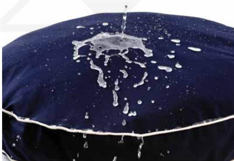
Water beads on fabric treated with nanotechnology from Schoeller Textil. Schoeller NanoSphere has been tested and certified safe by SUVA, says the company.
